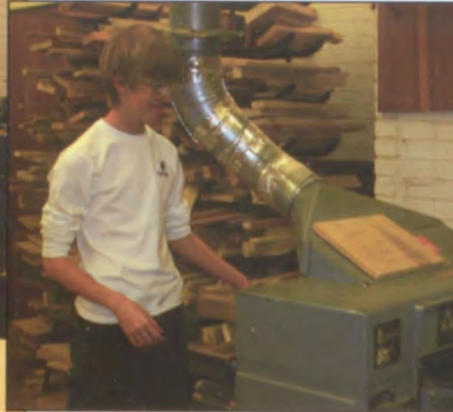
Adam Young using the planer to flatten the wood on both sides and shave it to its desired thickness.
