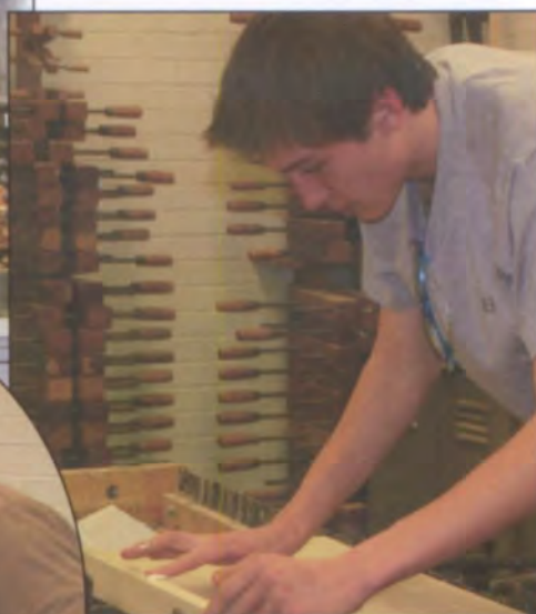
Grant Latus glues wood together to construct the body.
