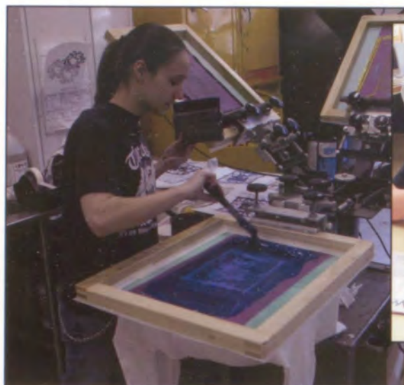
Danielle Sambrick creates a design on her shirt using a multicolor direct screen printing process. This involves putting ink on one side of the machine and then spinning it to do the same on the other.
